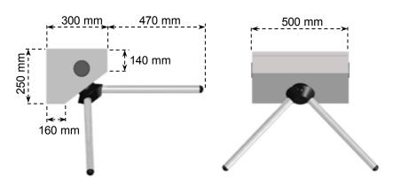
**Power Requirements** : 110/220V. 60/50Hz. AC (%±10) 24V. DC at standby ∼11W. max. ∼60W.
